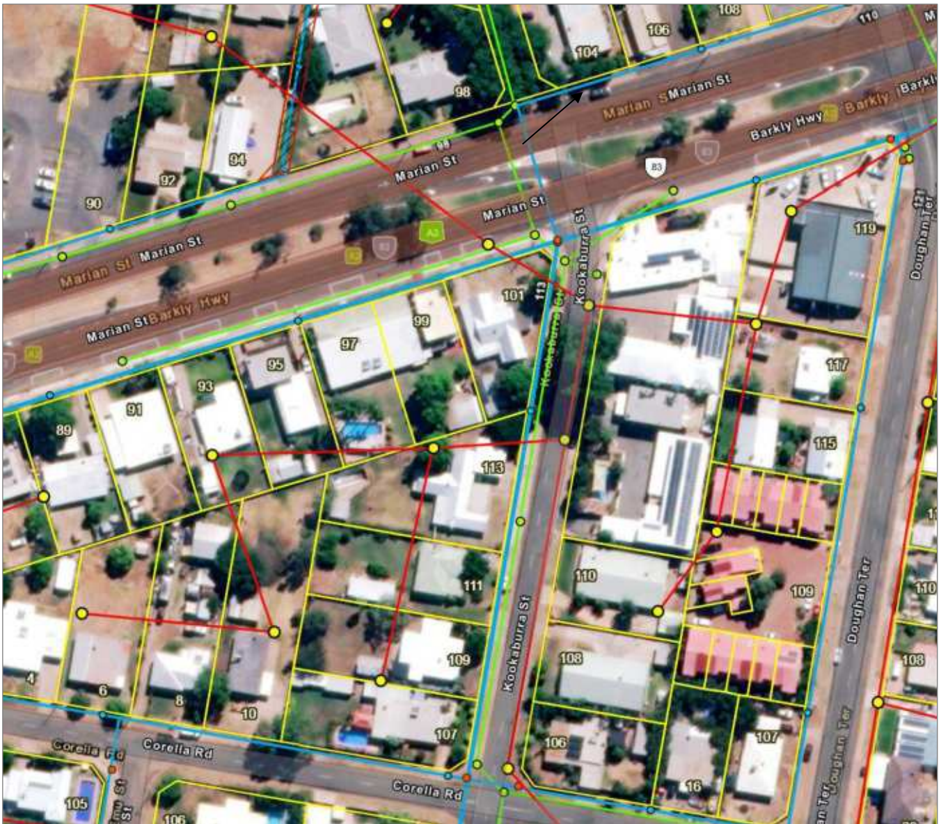
FIGURE 4 EXISTING STORMWATER NETWORK (M/C INFRASTRUCTURE MAPS 2023)
