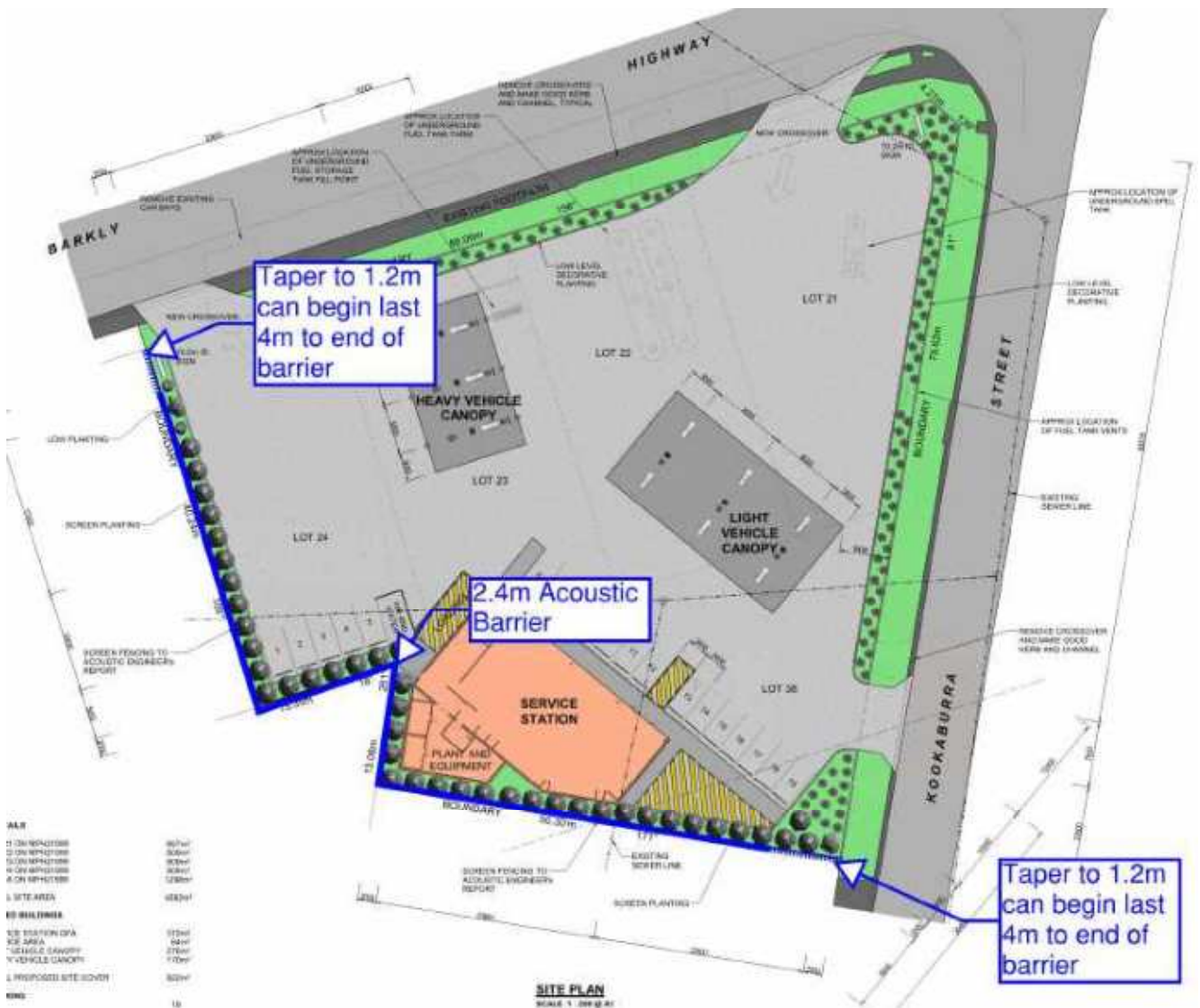
Figure 4 Acoustic Barrier Design
