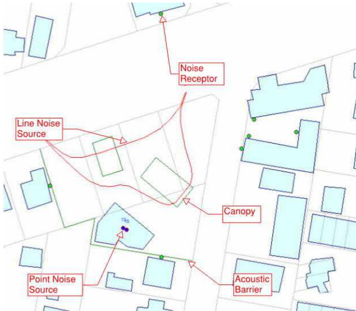
Figure 3 Noise Sources and Acoustic Barrier as Digitised into the Computer Model
