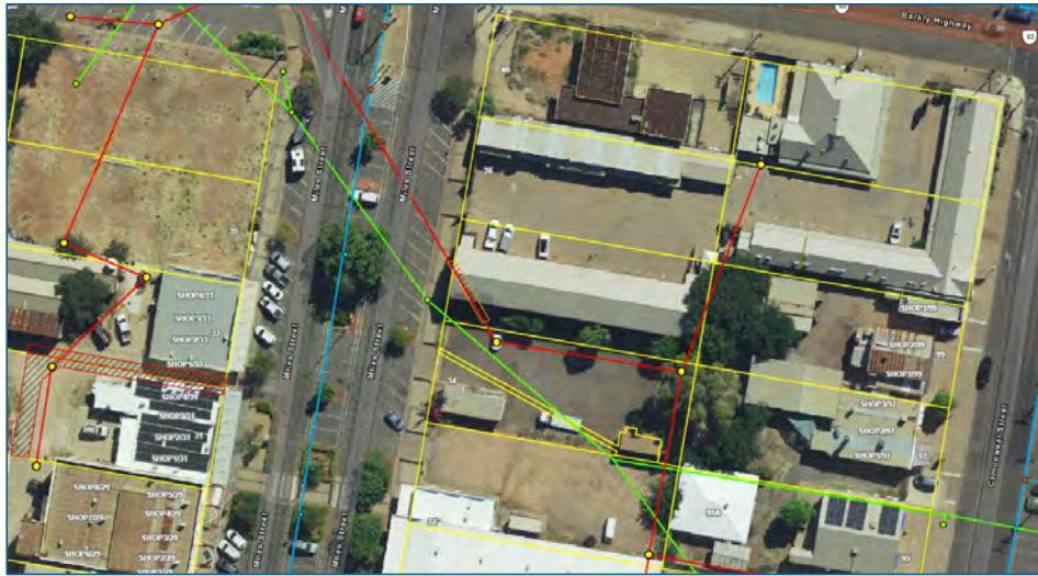
Figure 3- Site Plan indicate Sewer (Red), Stormwater (Green), Electricity Easement (Yellow), and 11Kv supply (blue)
