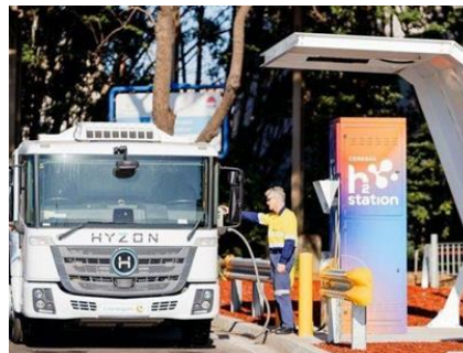
Figure 4-7: Representative hydrogen charging station
