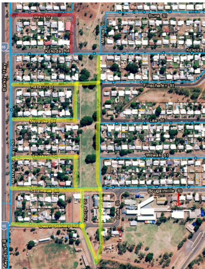
Figure 1 - Water main replacements
