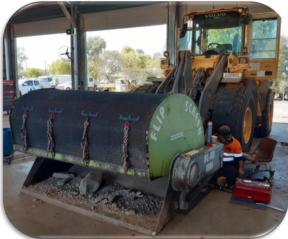
Figure 2: Works conducted on the Batch Plant Flip Screen attached to a Volvo Front Loader. The Volvo Loader also had a service upon arrival.
