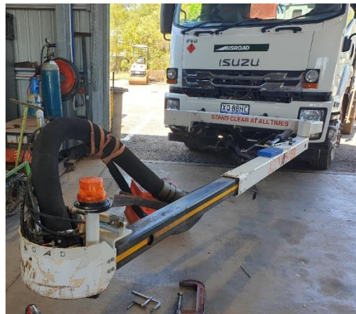
Figure 2: Repairs to Jet Patcher arm to improve on strength and structure.
